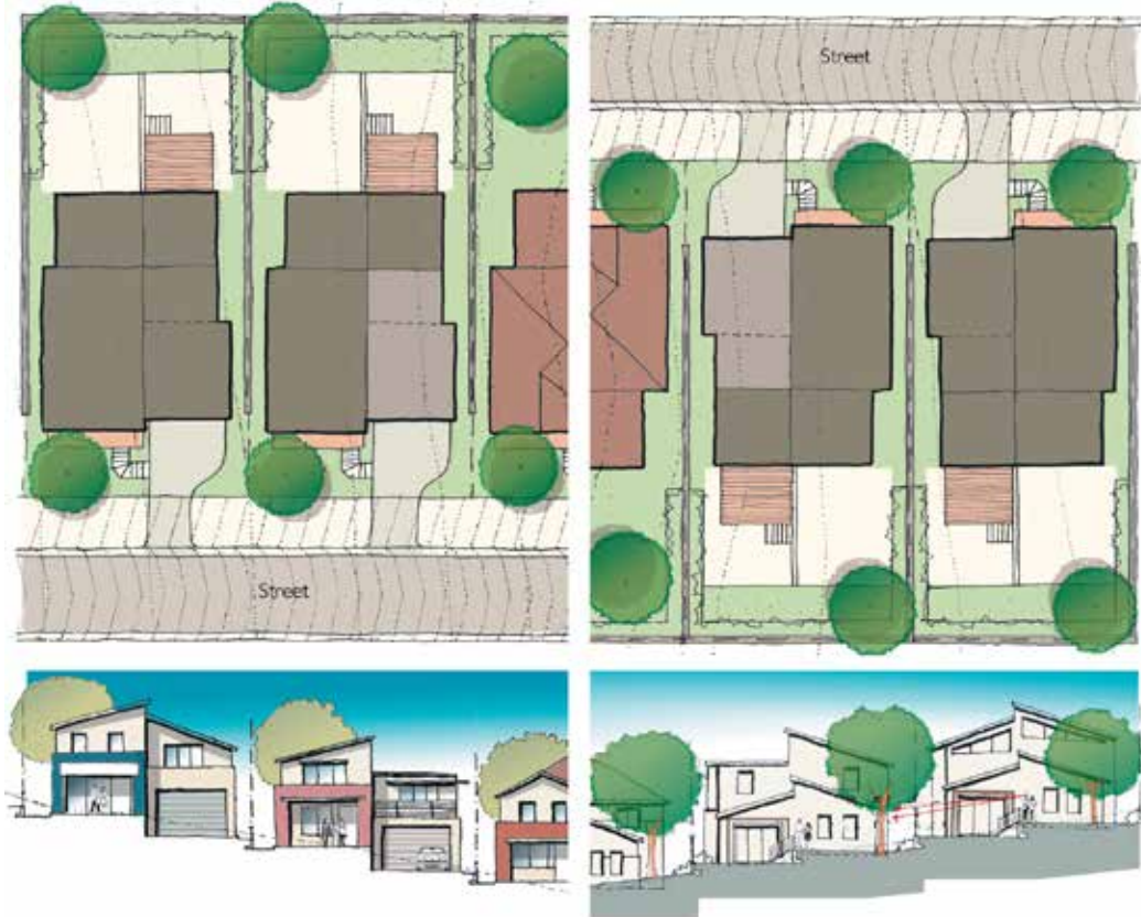
Figure 27: Split level house designs for cross slopes
