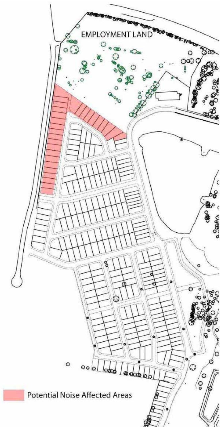
Figure 79: Area requiring acoustic treatment
