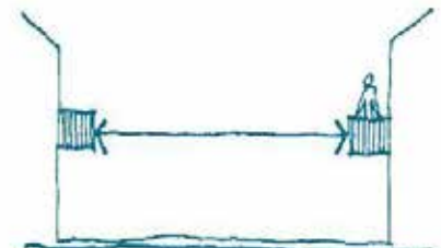
unscreened balcony separation
