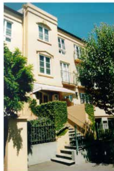
Figure 5.5 Each building should have a clearly defined entry. This example utilises both building form and its relationship with the street to clearly define the main entrance.
