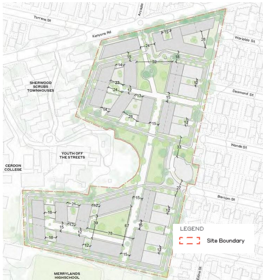
Figure 9: Building separation setbacks
