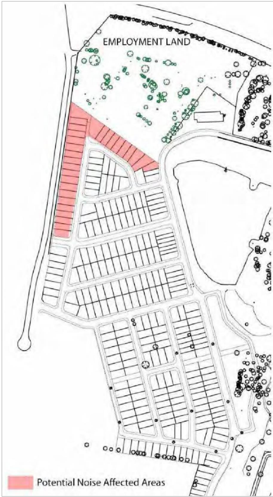
Figure 78: Area requiring acoustic treatment
