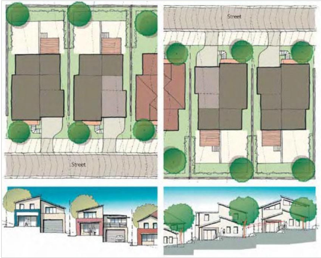
Figure 27: Split level house designs for cross slopes
